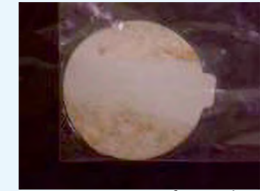
Appearance of sample (A smeared sample on the jig for removing deposits from X-2 penetration of Unit 1) (Approx.5cm in diameter)
